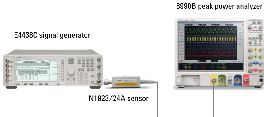
Figure 23-1 Test setup for the pulse characterization measurement
